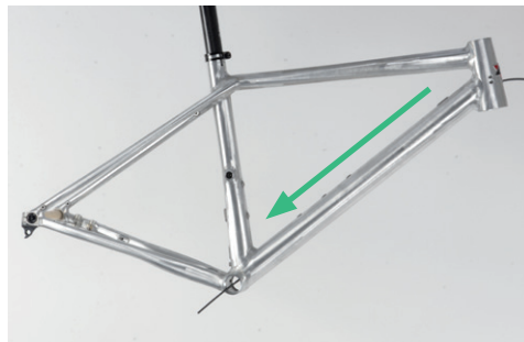
2. Have the cable exit the frame at the right-hand side next to the bottom bracket.
