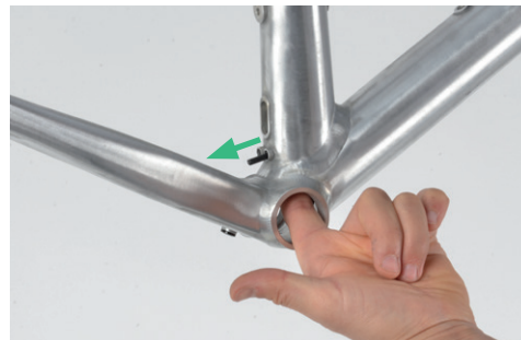
5. The shifting cable housing is to be guided towards the top end hole of the seat tube. Push and pull it – from the top and the bottom – simultaneously.
