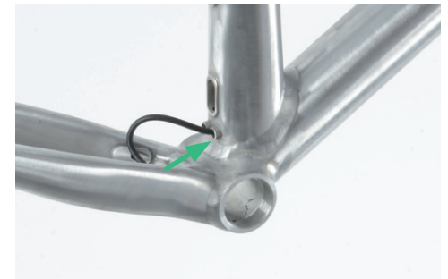
9. Push the cable housing at the steering tube and simultaneously guide the looping backwards. Make sure, the cable housing is not bent.
