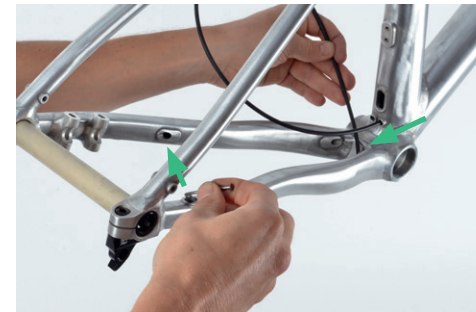
7. Push the one end of the cable housing into the chain stay until it can be seen at the rear end of the right-hand chain stay. Guide it out of the chain stay using a nail, for example, and have it exceed the chain stay with approximately 20 cm.
