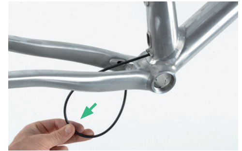
8. Twist the looping downwards in order to prevent the cable housing from breaking off.
