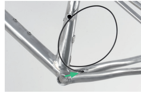
6. Form a looping with the cable housing and insert it into the right-hand chain stay.
