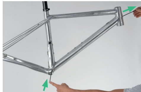
4. Pull the shifting cable housing including the foam tube back and bend the end of the cable.
