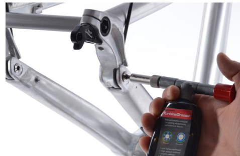
Picture shows bearings that can be greased at the HorstLink.
