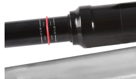
The illustration shows the SAG indication on the damper.
