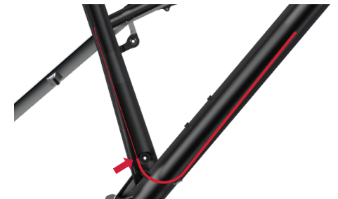
Picture shows rear brake on Post Mount socket with hose routing for SRAM.
