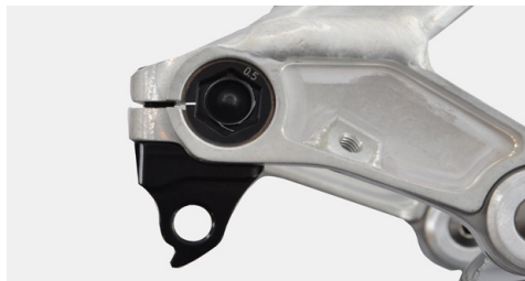
The picture displays the insert and the clamping notch aligned correctly.
