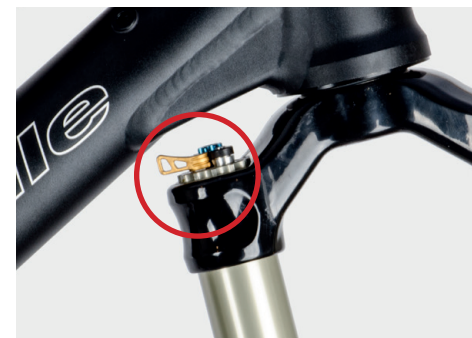
Illustration: Clearance at the down tube
