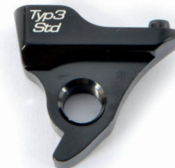
Illustration. 05: Std. rear derailleur hanger for Shimano-Shadow and SRAM.
