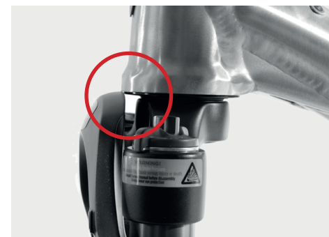
Illustration: Clearance at the steering tube
