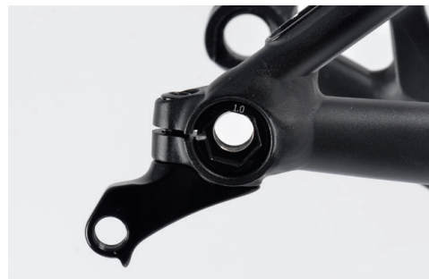
Illustration: The picture displays the insert and the clamping notch aligned correctly.
