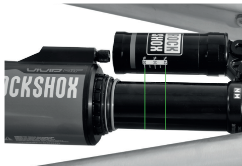
The picture shows SAG measurement on the damper.
