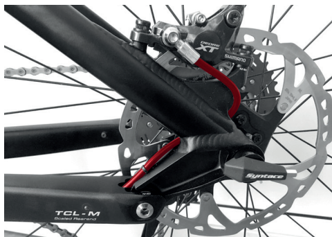
Picture shows rear brake on a Post Mount socket with hose routing for Shimano.
