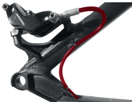
Picture shows rear brake on Post Mount socket with hose routing for SRAM.
