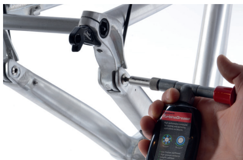
Picture shows bearings that can be greased at the HorstLink.
