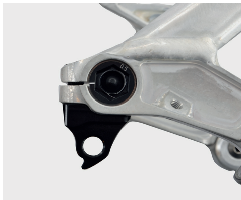
The picture displays the insert and the clamping notch aligned correctly.
