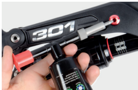
Picture shows bearings that can be greased in the top tube.
