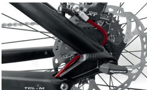
Picture shows rear brake on a Post Mount socket with hose routing for Shimano.
