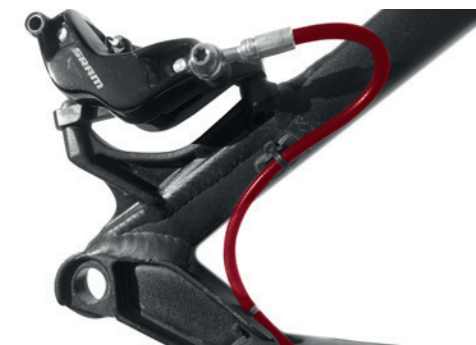
Picture shows rear brake on Post Mount socket with hose routing for SRAM.
