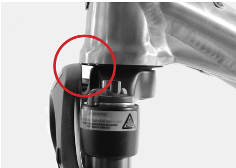
Illustration: Clearance at the steering tube
