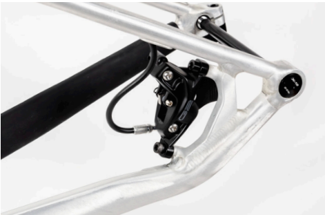
Illustration: Brake caliper mounted on PM standard socket with SRAM components.
