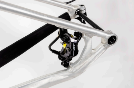
Illustration: Brake caliper mounted on PM standard socket with Shimano components.
