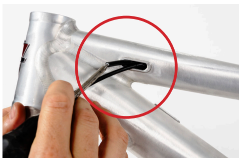
Illustration: Exit of the brake hose at the top tube.
