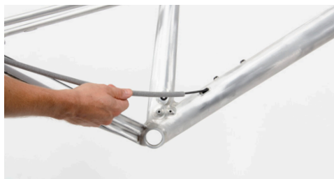
Illustration: Inserting the foam tube
