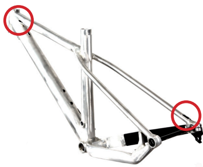
Illustration: cable housing rear derailleur insert and exit.
