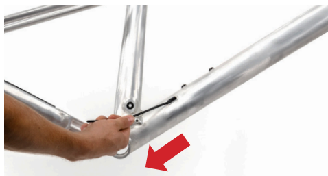
Illustration: pulling the housing out of the down tube above the bottom bracket
