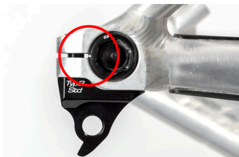
Illustration: The picture displays the insert and the clamping notch aligned correctly.
