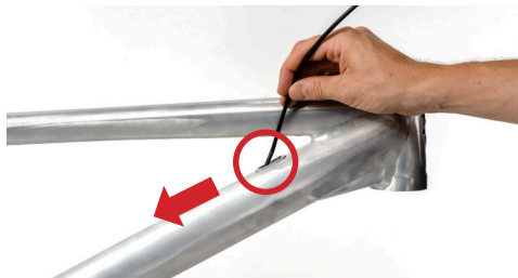
Illustration: inserting the housing in the down tube.
